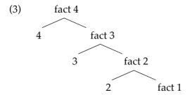
Note that the hierarchical structure directly stems from the fact that the implementation is underlain by a two-equation system: A variable plus a self-call, and it is the latter that expands into the base case, effectively terminating the recursion and the overall computation. It is this specific characteristic that explains why this type of hierarchy, a binary tree, automatically results from a recursive implementation.
